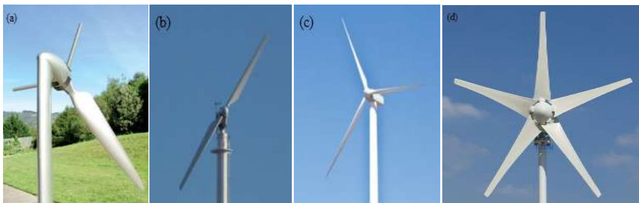
Figure 2.4: Types of HAWT (a) single-blade (b) double-blade (c) three-blade (d) five-blade [19]
