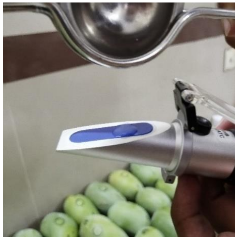
Figure 3: Measuring soluble solid content with refractometer
