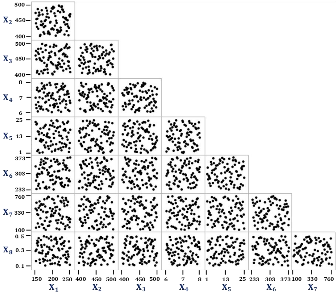
Figure 3.1: Design space to conduct computer experiment for MEMS accelerometer optimization.
