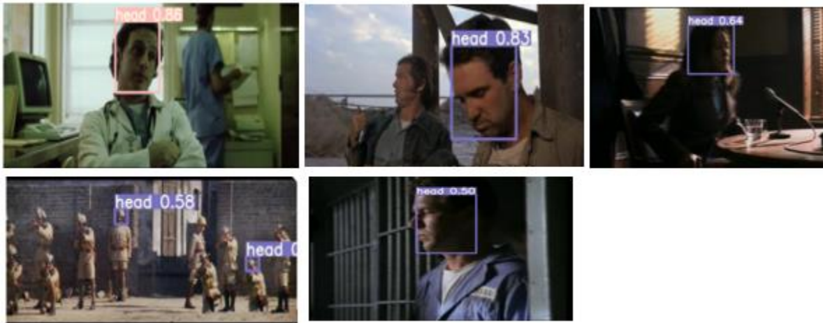
Figure 15: Head detection results using dataset for training Casablanca dataset on yolov5 and testing Hollywood Heads dataset
