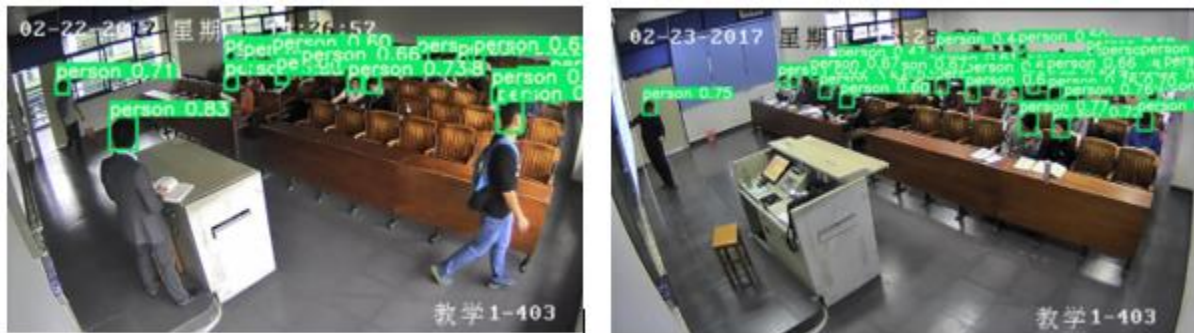
Figure 23 Head detection results using Scutheads dataset for training and ScutHead dataset for testing on yolov5
