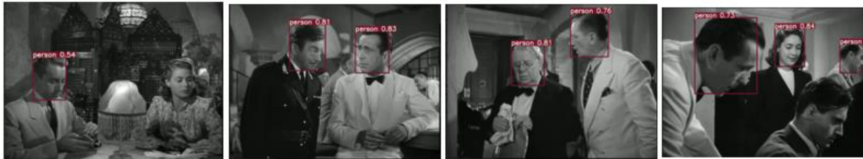
Figure 25: Head detection results using Merge Dataset for training and Casablanca dataset for testing on yolov5
