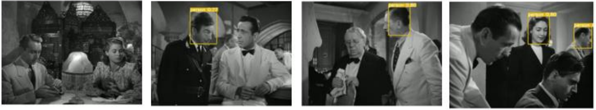
Figure 18: Head detection results using Hollywood heads dataset for training and Casablanca dataset for testing on yolov5
