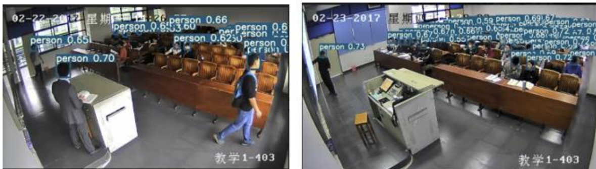
Figure 27: Head detection results using Merge Dataset for training and ScutHead dataset for testing on yolov5
