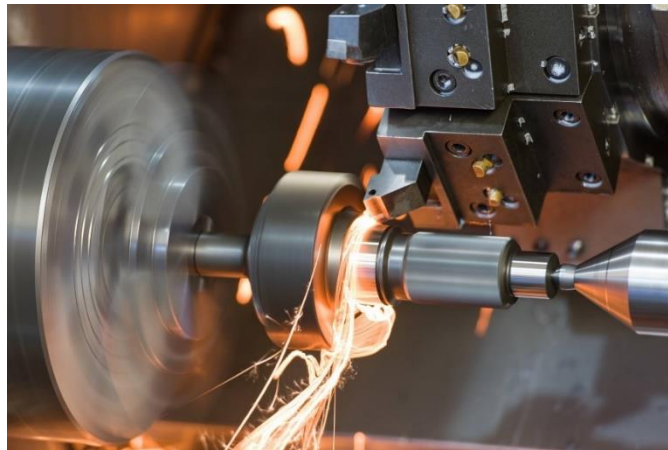
Figure 9: Material undergoing a machining process on CNC Lathe [24]
