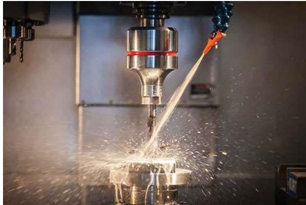
Figure 15: Ultrasonic Machining being done[28]
