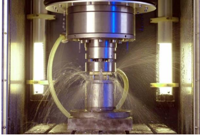
Figure 16: Electrochemical machining being done [29]
