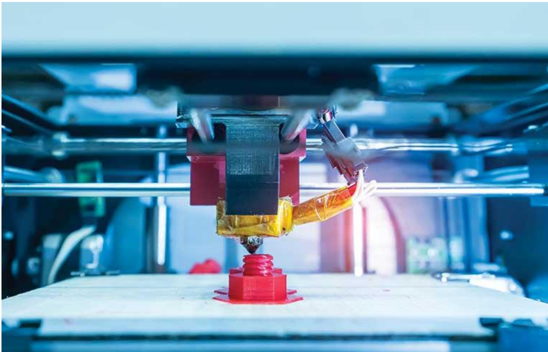
Figure 8: 3d printing of a bolt being done [23]
