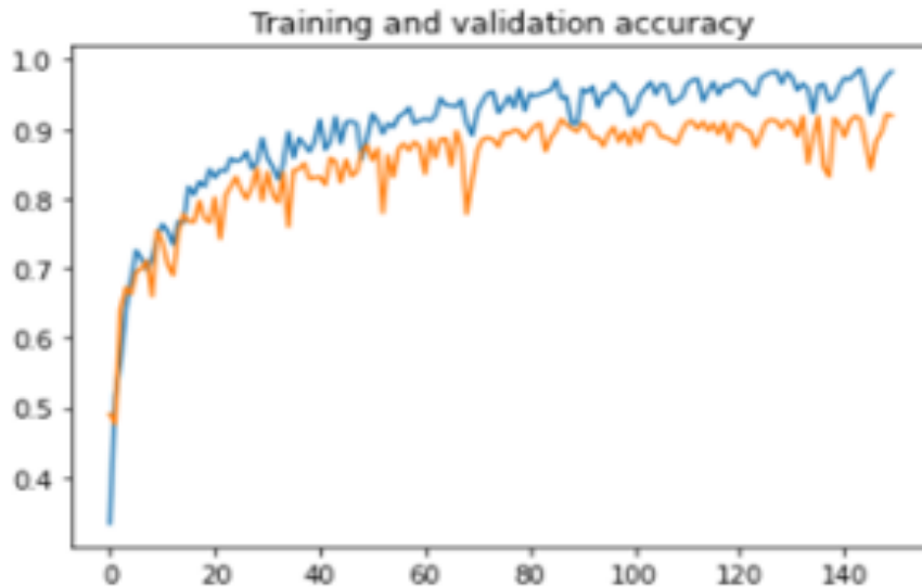
Figure 5.2 Graph for accuracy against each epoch of MobileNetV2
