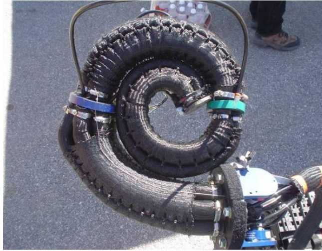
Figure 15 Oct arm made by parallel linear actuators [19]
