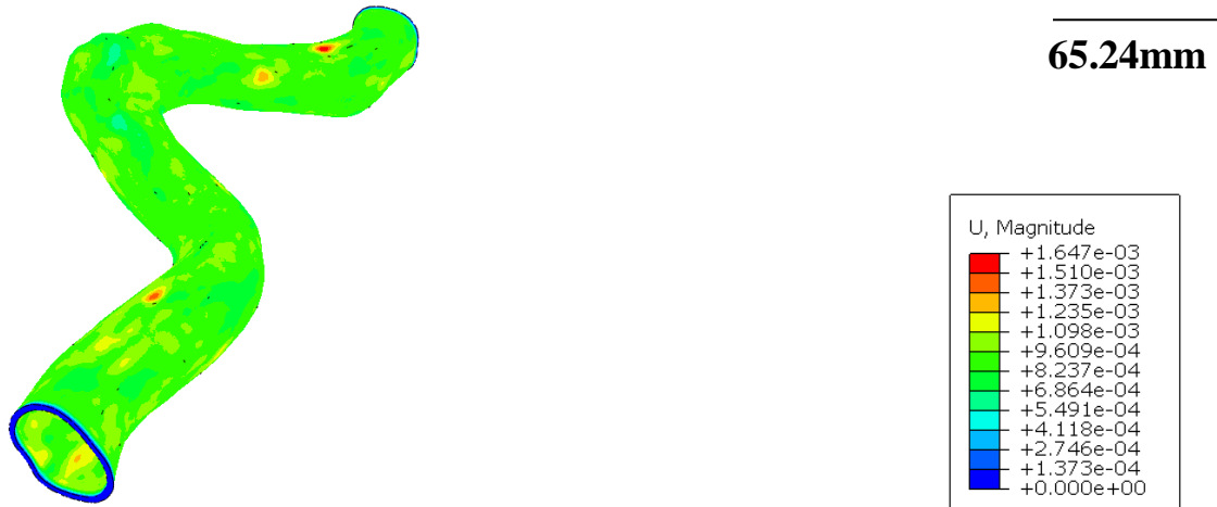
Figure 4.13: Deformation (U) Plots on Healthy Model showing distributed deformation using Structure based approach.
