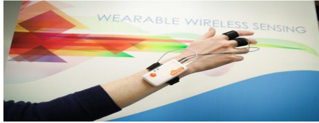
Figure 13 Placement of Shimmer GSR unit on finger [38]
