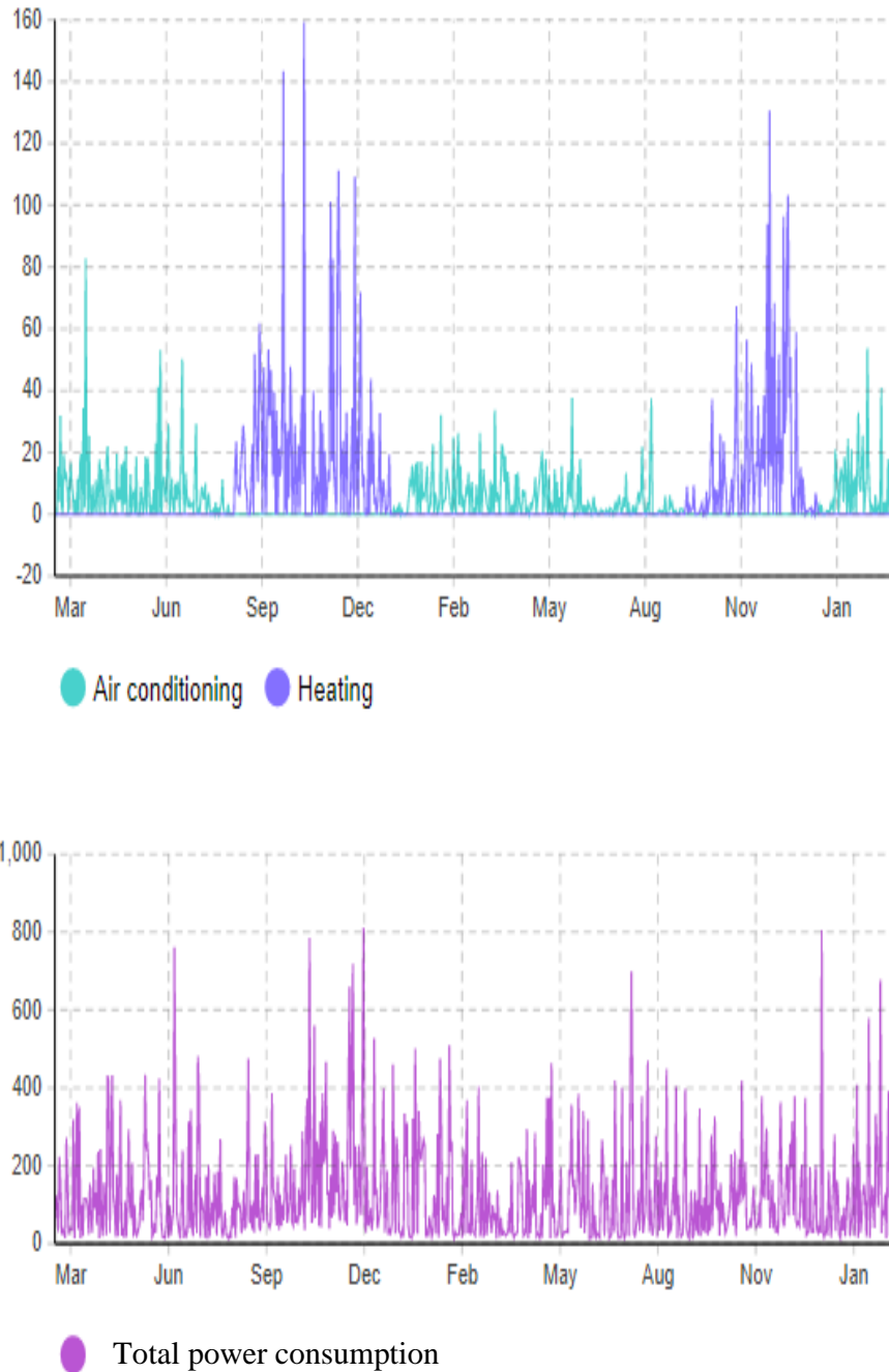
Fig. 5.7: Impact of climate on A/C, heating, and total power consumption
