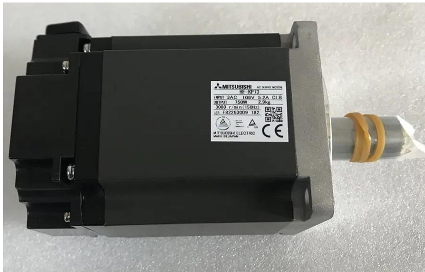
Figure 28 HF-KP73 AC servo motor for vertical motion of carriage
