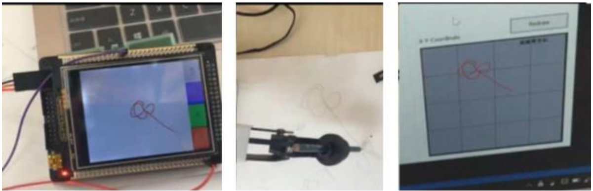
Figure 19 Touchscreen for input, end-effector tracking and attached computer screen [24]
