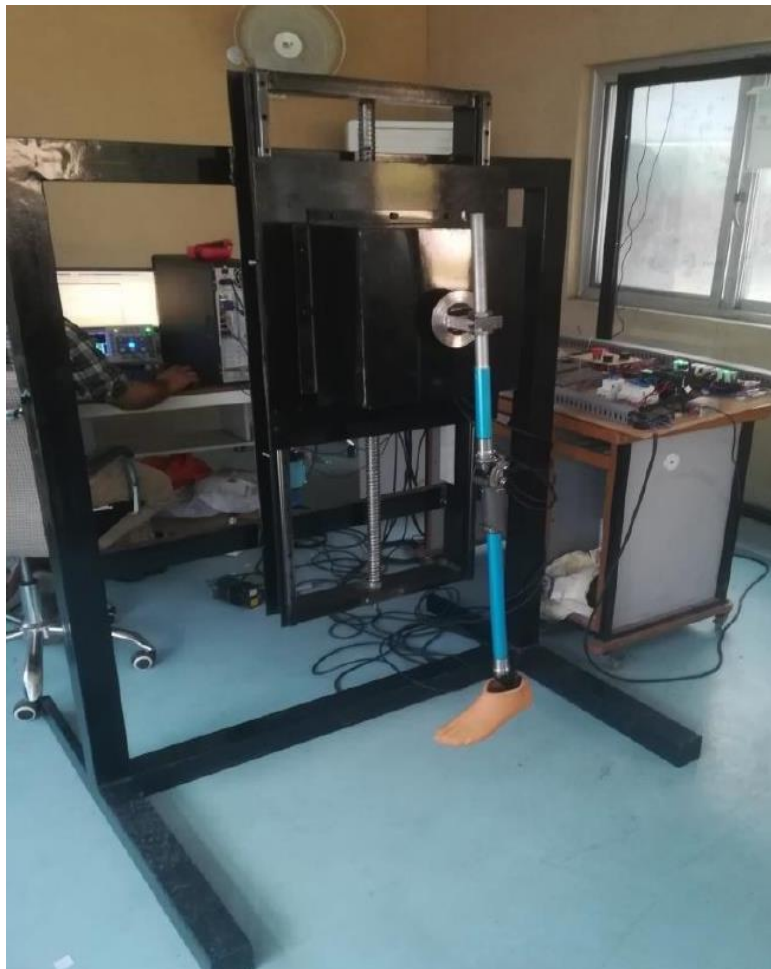
Figure 27 Prosthetic testing platform
