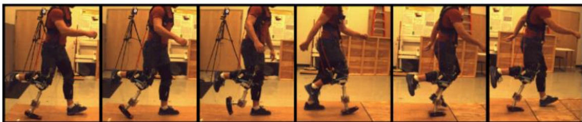
Figure 2-9 Walking Gait of prosthesis mounted on able-bodied using able-bodied testing adaptor [40]
