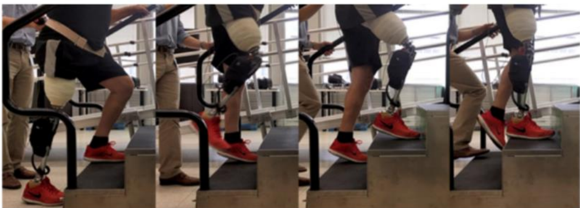
Figure2-8 Transfemoral Prosthesis Attached to Above knee amputee during step climbing test[39]
