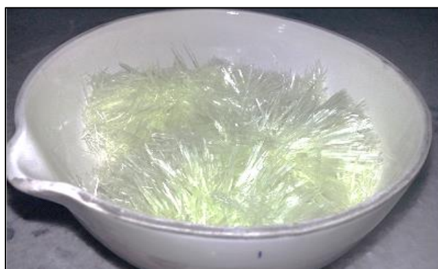
Figure 13. Needle shaped crystals of dinitrobenzene.
