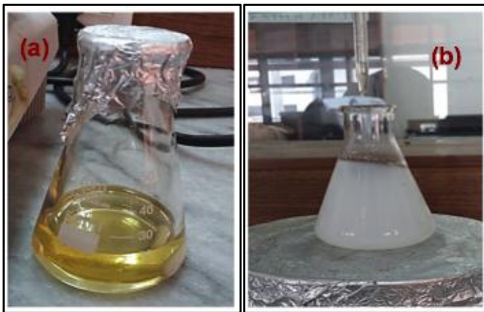
Figure 3.1 (a) TTIP + propanol solution, (b) Drop-wise addition to H 2 O+HNO 3 solution
