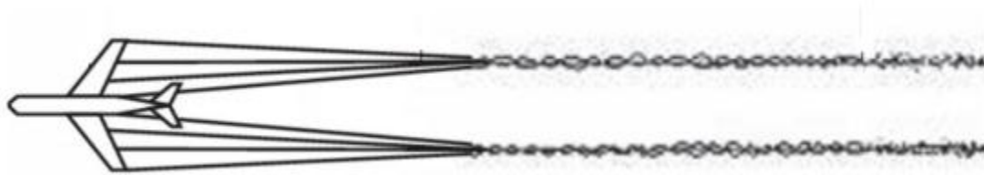
Figure 3.1: Aircraft Vortex System [8].
