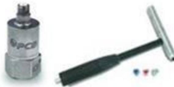
Figure 4.5 - PCB Accelerometer and Impact Hammer for Measuring Vibration
