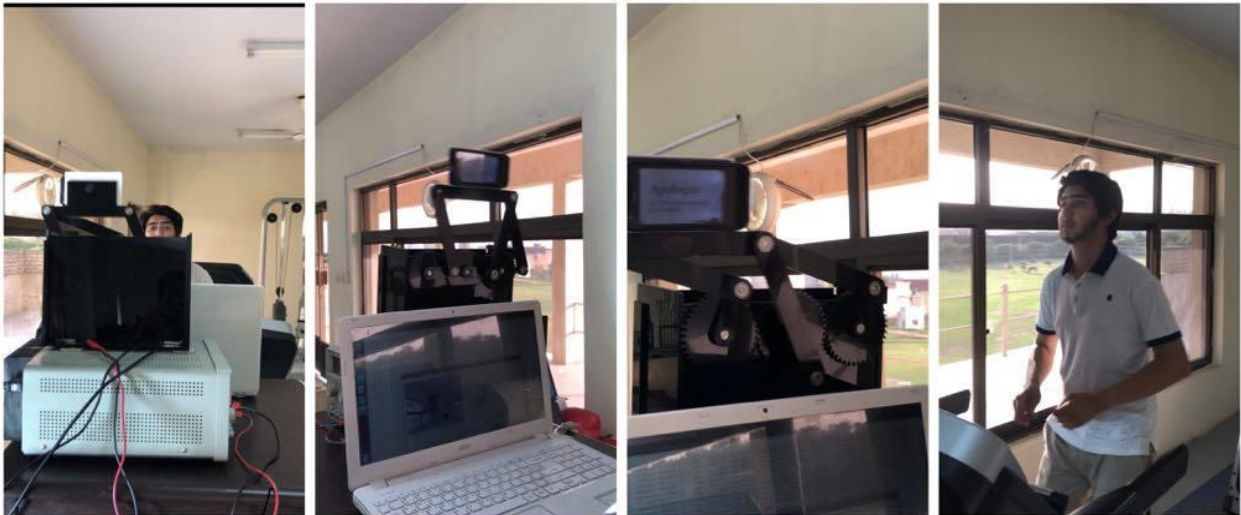
Figure 14: Experimental Setup: the platform is placed stationary in front of the user at a fixed distance from the treadmill
