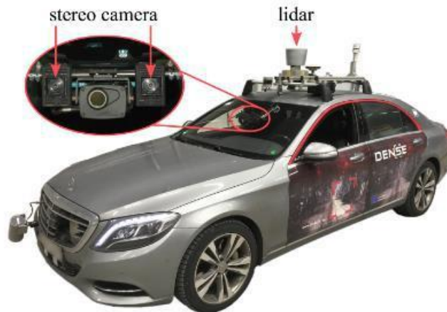
Fig 3.0 Test vehicle equipped with a RGB stereocamera (Aptina AR0230, 1920x1024, 12bit) and a lidar(Velodyne HDL64-S3, 905nm)
