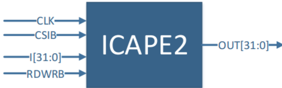
Figure 19: ICAP primitive for 7-series FPGA devices
