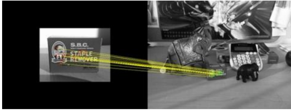
Figure 2.5: Object detection (left) in a cluttered scene (right) using a combination of feature detection, feature extraction, and matching
