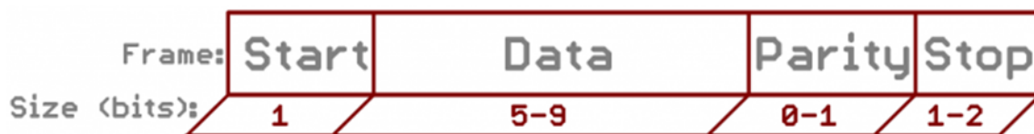
A serial frame. Some symbols in the frame have configurable bit sizes.
