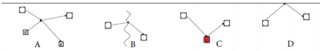
Figure 1.4 Illustrate scattering mechanisms of phonon-electron scattering, phonon-defect scattering, phonon-phonon/impurity scattering and phonon-boundary scattering respectively
