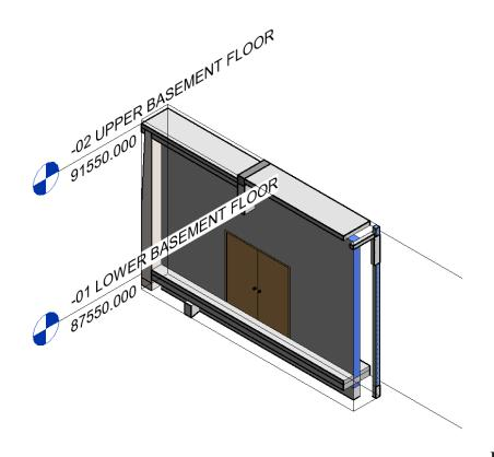
This is the part of the design which has a clash detected in it. Now we can resolve the clash by altering the design in Revit which will reduce the quantity of the material used in the model.
