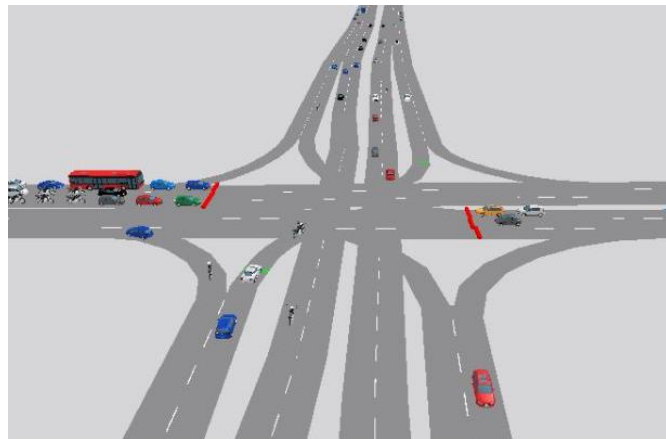
Figure 22 Vissim model of SPUI
