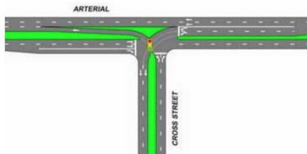
Figure 9 Continuous Green T-Intersection
