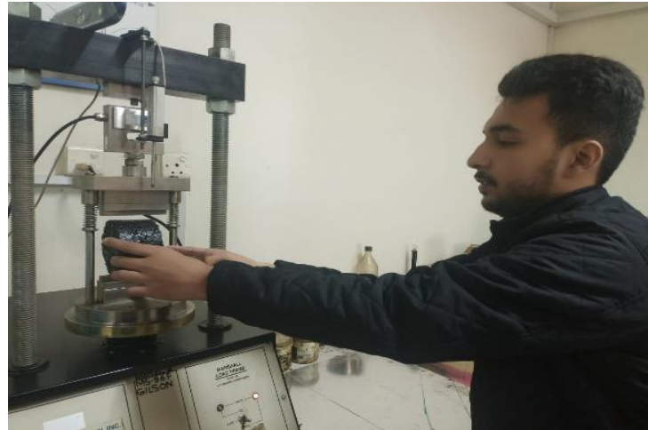
Fig 3.11 (Performing ITS Test)
