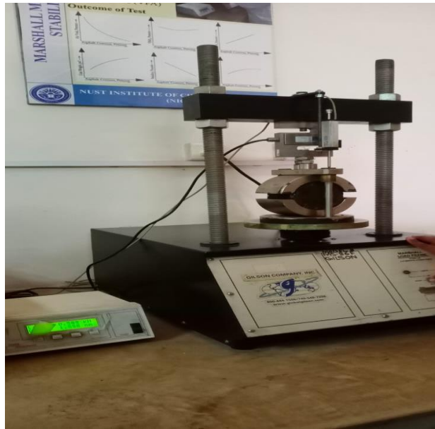
Fig 3.8 (Marshall Test Equipment)
