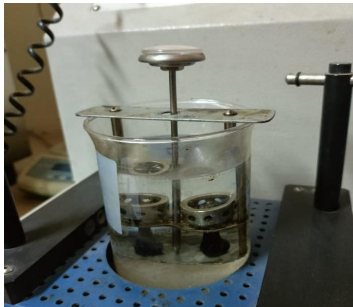
Fig 3.6.1 (Softening Point Test Equipment)
