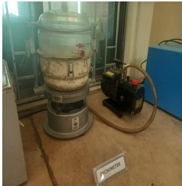
Fig 3.10 (Gmm Test Equipment)
