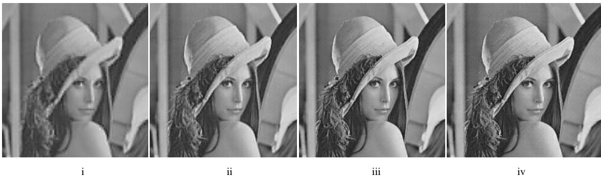
Figure 17: Lena Image (i) Reconstructed Image From the 10% DCT coefficients estimated by MLP Model (ii) Reconstructed Image From the 25% DCT coefficients estimated by MLP (iii) Reconstructed Image From the 45% DCT coefficients estimated by MLP (iv) Reconstructed Image From the 100% DCT coefficients estimated by MLP
