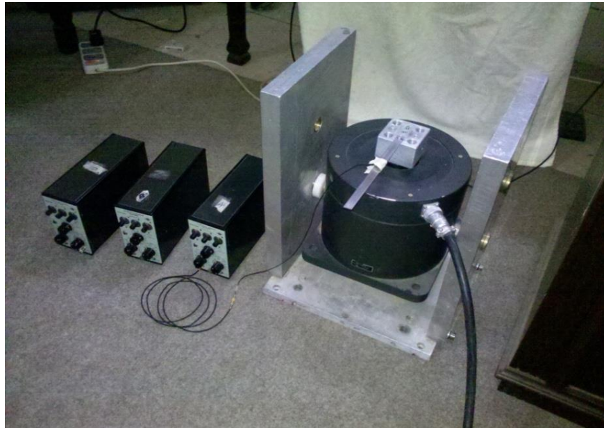
Figure 3-7: Setup to find Natural Frequencies
