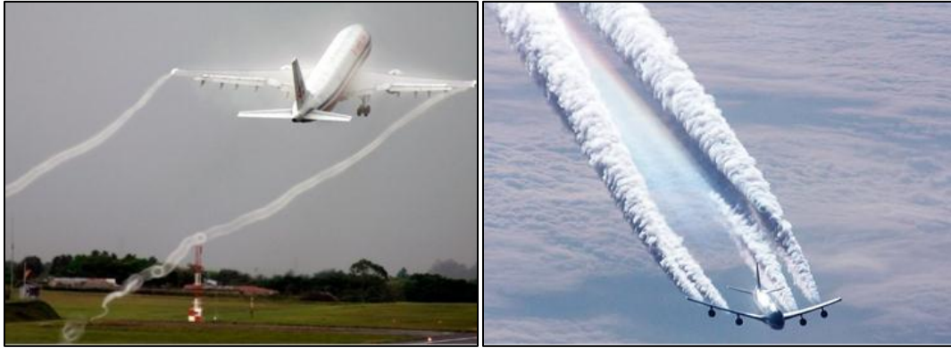
(b) Contrails behind a Boeing 747 engines entrained by wingtip vortices (air-liners.net)
