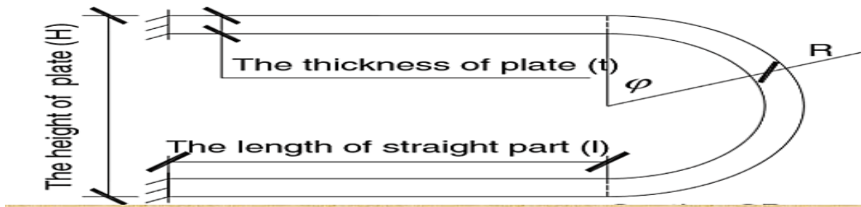
Figure 35: Dimensions of U-Shaped steel plate
