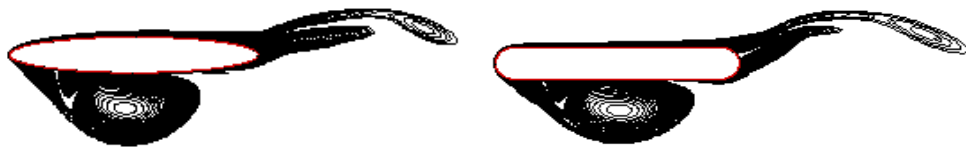
Figure 5-11 Vorticity plots at maximum value of drag coefficient
