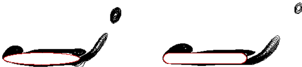
Figure 5-13 Vorticity plots at minimum value of drag coefficient
