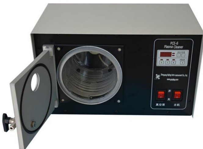
Figure 3.3. Image of plasma cleaner instrument
