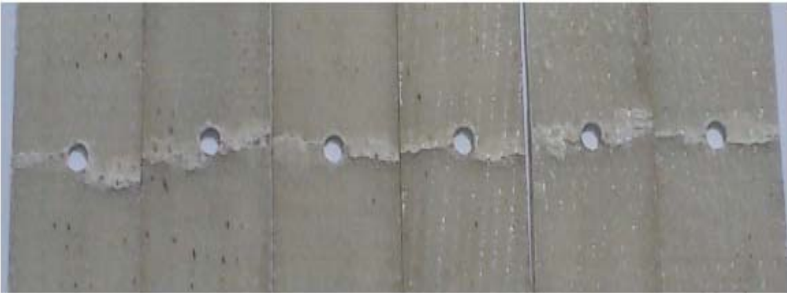
Figure 46: Damaged specimens of 3D woven GFRP composites-A zoomed view
