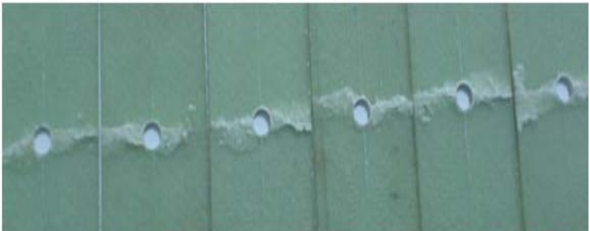
Figure 44: Damaged specimens of 2D woven GFRP composites-A zoomed view
