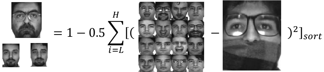
Figure 13: RNCC failed with the whole image (holistic) for occlusion with scarf and glasses.
