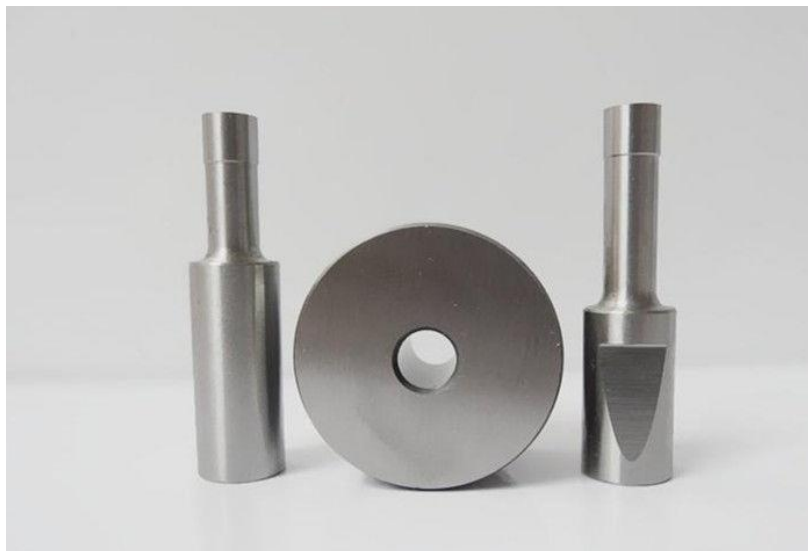
Figure 6. Manual die with upper and lower punch, size 2
