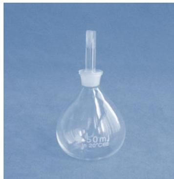
*Figure 1.10: Specific gravity bottle.*
