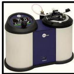
*Figure 1.12: Close cup flash point tester.*
