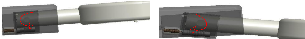
Fig.13 Wrist rotating motion, (i) counter clockwise motion, (ii) clock-wise motion.
