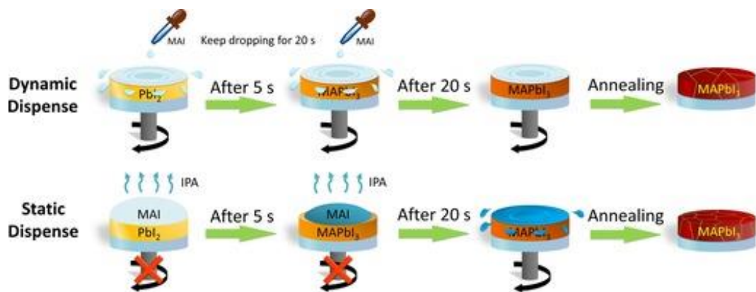
Figure 3.3: Process of Static & Dynamic Spin Coating [5]
