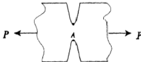
Figure 5: Case 2 - Axial tension P = 40\text{N} applied to opposite V notches in finite width plate
