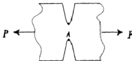
Figure 6: Case 3 - Axial tension P = 100\text{N} applied to opposite V notches in finite width plate
