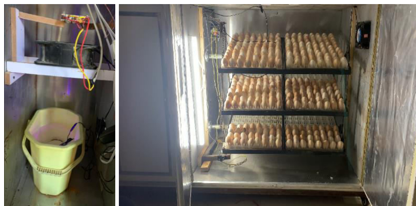
Figure 3.2: (a) Heating Chamber (b) Main Chamber for Incubating Eggs
