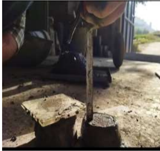
Figure 4.3: Deformation test under 500g loading.
