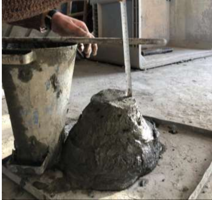
Figure 4.2: Slump cone test to measure the slump of concrete.
