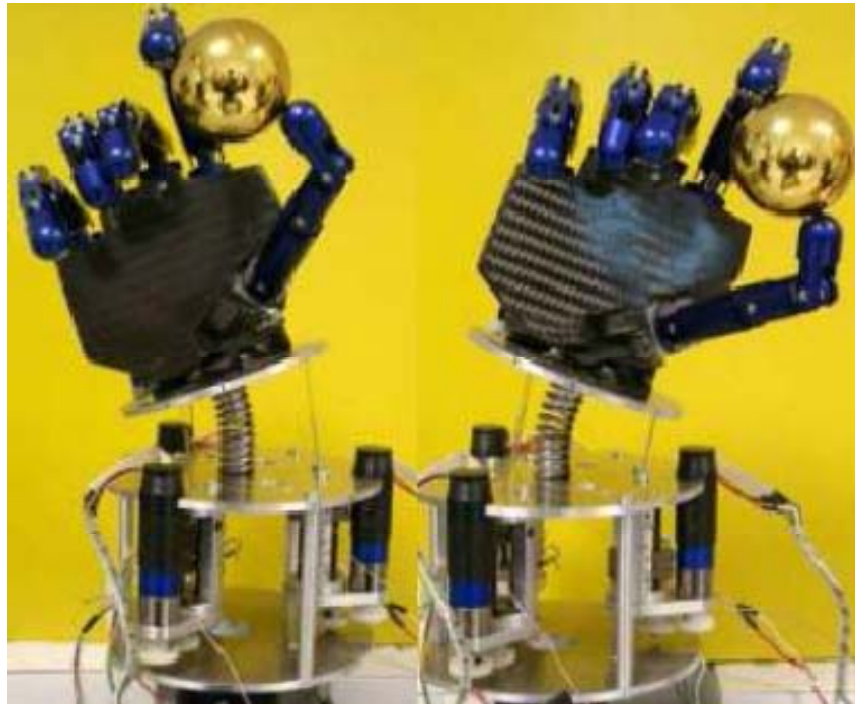
Figure 11: Prototype trials of ARTS Wrist: on the right Adduction and on the left Abduction
