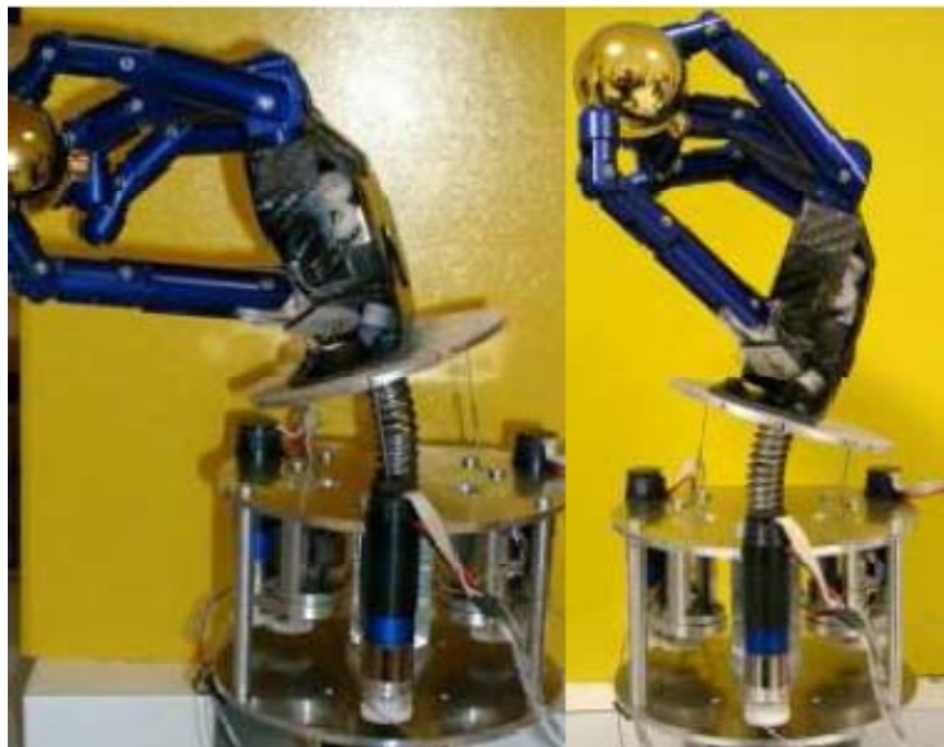
Figure 12: Prototype trials of ARTS Wrist: on the left Flexion and on the right Extension
