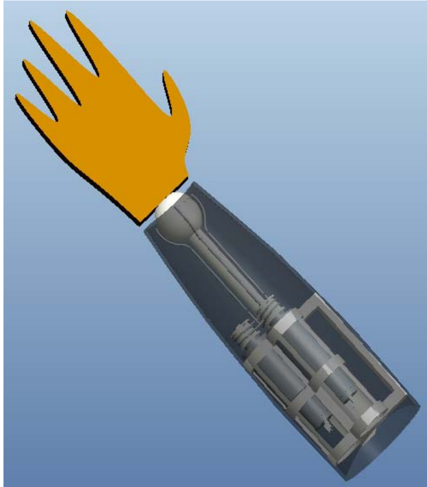
Figure 28: Pro-E model of the wrist actuator with forearm casing.
