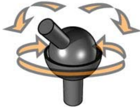
Figure 20: Ball & Socket Joint with three rotations indicated
