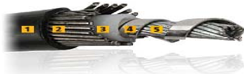
Figure 27: Construction of Bowden cable 1) plastic sheathing 2) outer sheathing made of spring steel wire 3) Teflon guide sleeve 4) spiral wire 5) inner core made of spring steel wire
