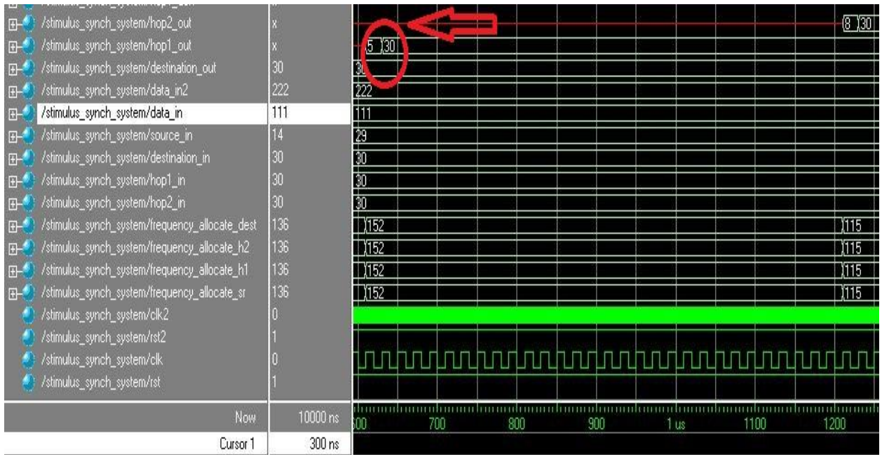
Figure 4.19 Hop-1 radio requests are transmitted by the Source radio during the next 30 time slots of the super frame.
