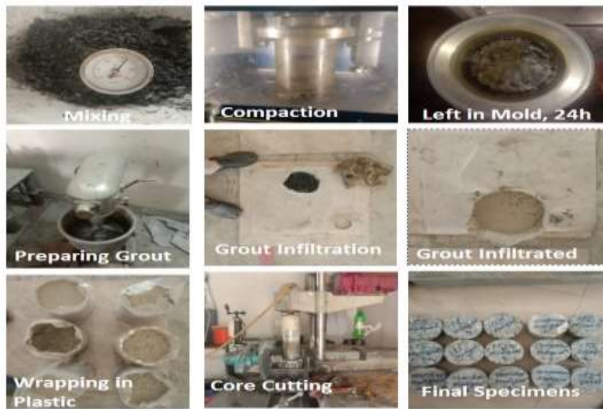
Figure 3.19 Preparation of semi-flexible specimens
