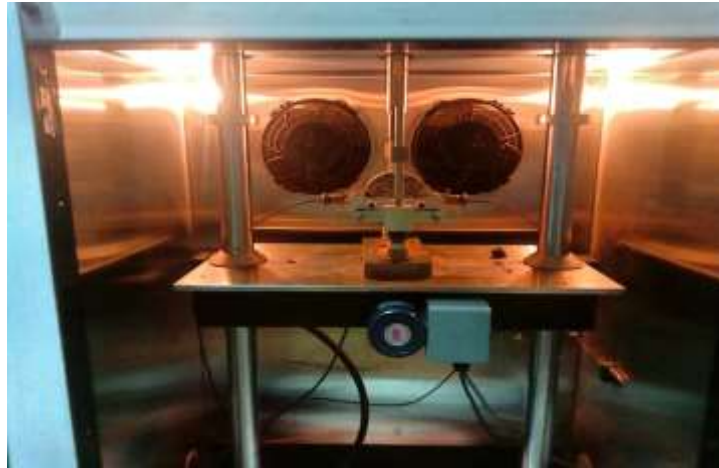
Figure 3.22 ITSM testing and sample positioning
