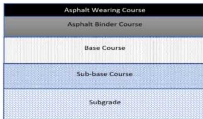
Figure 2.1 Components of flexible pavements
