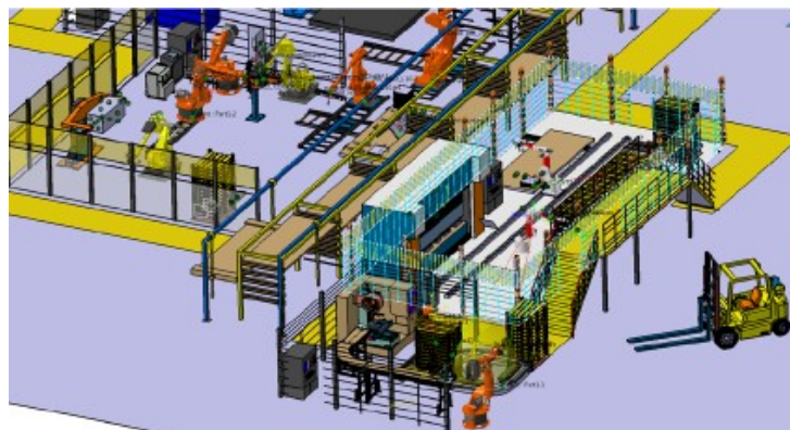
Figure 2: An example of FMS Plant 3 .
