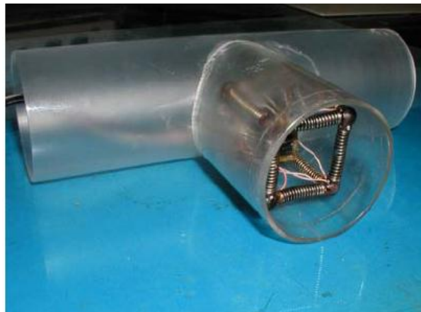
Figure 19, Design of linear SMA actuator [8]
