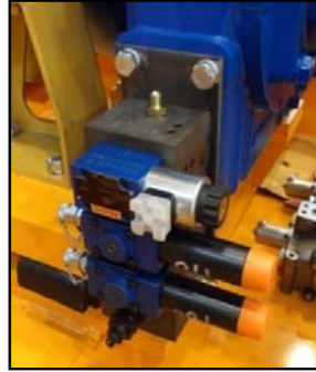
Fig 6.1: Old/Existing hydraulic Circuit Valves and Manifold
