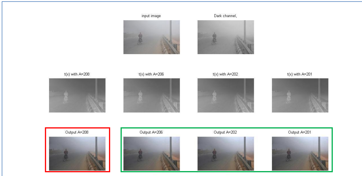
Figure 5.7 Image Restoration with Improved Atmospheric Light Value – Dense Fog
