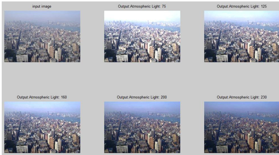
Figure: 5.4 Effect of Atmospheric light value – Normal Fog
