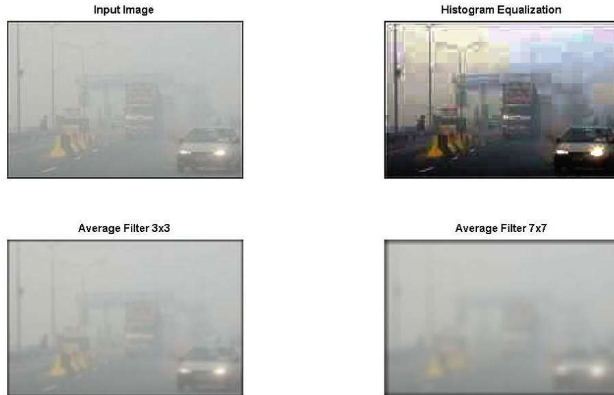
Figure 5.2 Foggy Image and Classical Image Enhancement, Histogram Equalization and Average Filter
