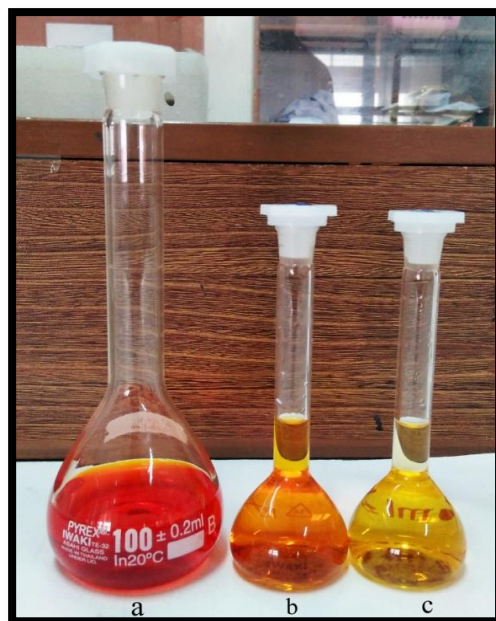
Figure 4.11 Different concentration solutions of methyl orange. (a) 3 mM, (b) 0.1 mM, (c) 0.01 mM.
