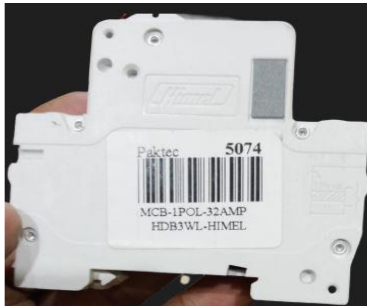
Figure 15 Single Pole Circuit Breaker
