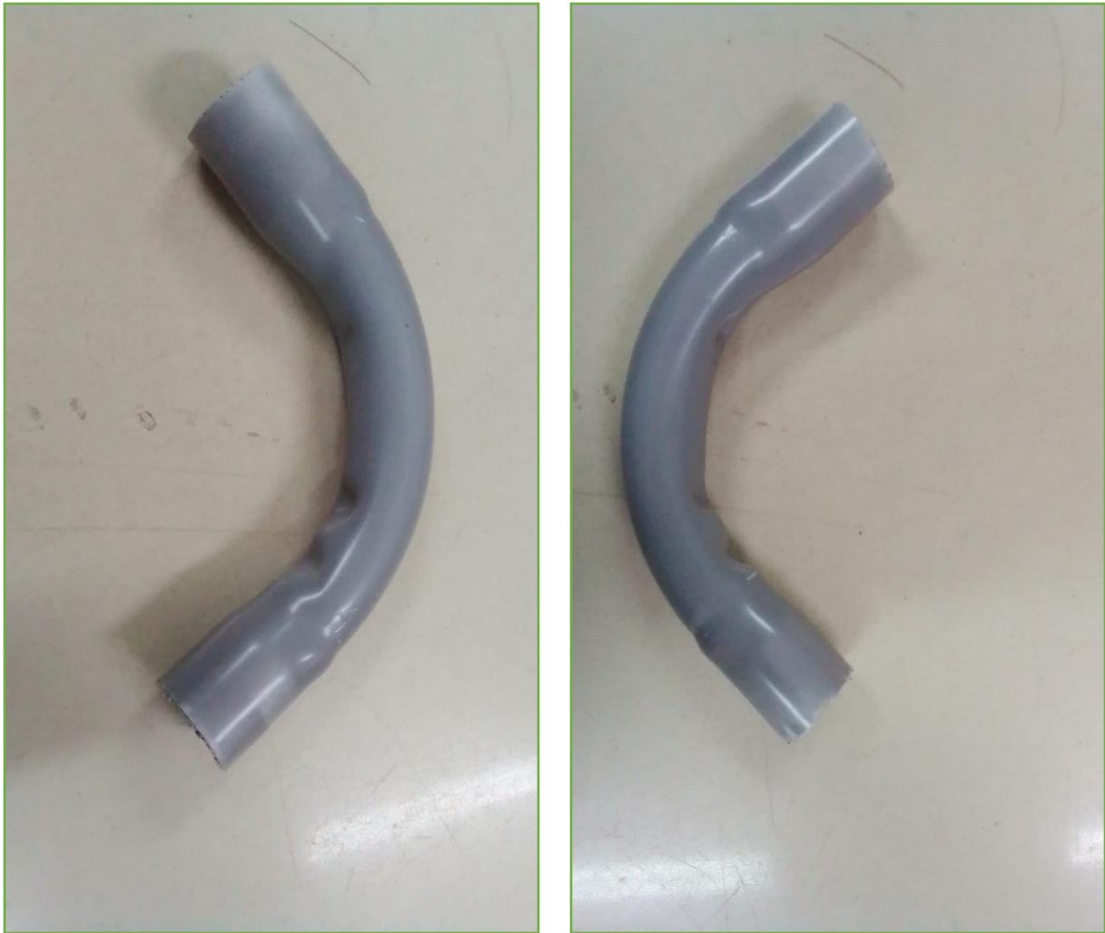
Figure 51 Poor Quality Pipe Samples without Air Blow
