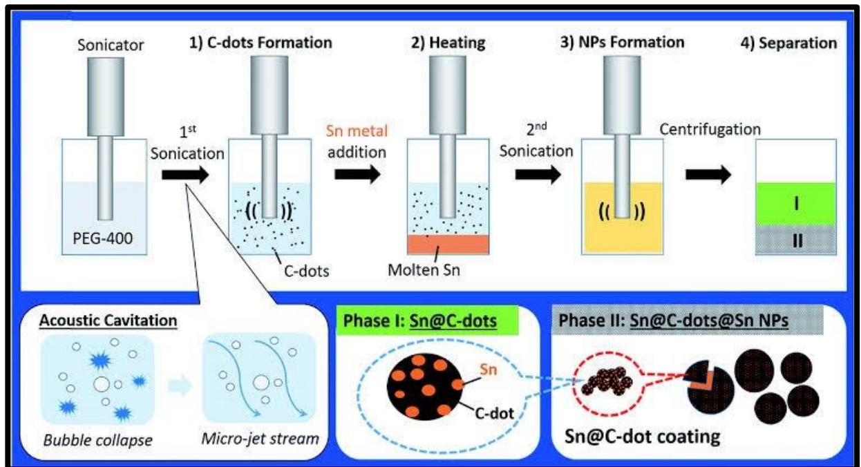
Scheme 2: Synthesis of Sn-C-dots nanoparticle via sono-chemical method [42]
